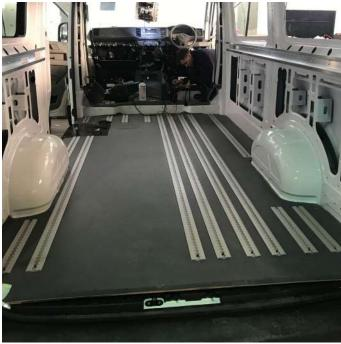
First clean the van floor and use primer on underside of the composite floor.
