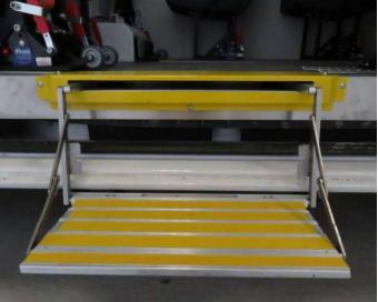
For M1 Ultra Lite flooring we can supply and fit a supplier side step to sit inside the floor.
