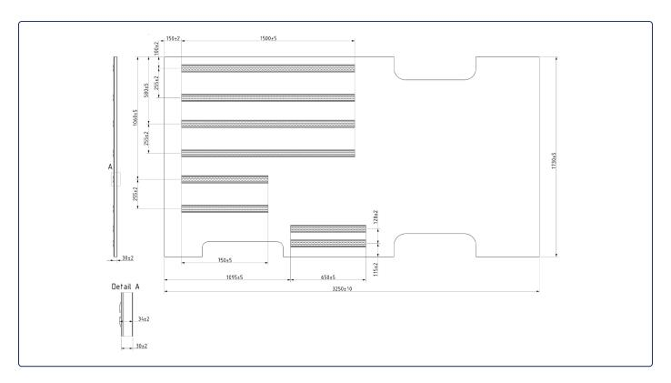
The floor is supplied in one single piece with rails, the wheel arches cut out and floor vinyl fitted. Flooring is supplied exactly to a drawing supplied following a discussion with the end user customer.
