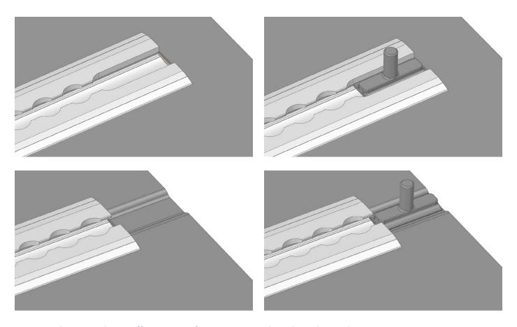
For use with NMI T Bolts we offer 2 options for insertion into the rails, as shown above.
