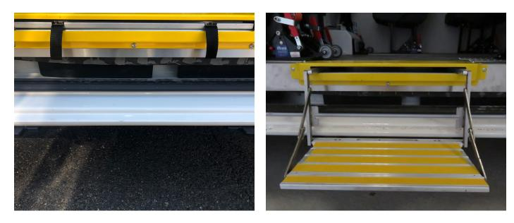
For M1 Ultra Lite flooring we can supply and fit a supplier side step to sit inside the floor.
