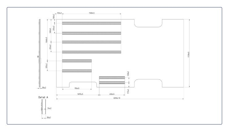
The floor is supplied in one single piece with rails, the wheel arches cut out and floor vinyl fitted.
