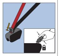
Once clips are at the bottom they can be locked by pushing the two larger ends together. These will make the belt straps feel less tight for the user. The passenger is now secure
