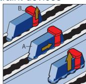
To remove the reel and stalk features pull up Plunger B, slide Plunger Stud Fitting A till the unit aligns with the holes in the track. When aligned the device can be lifted out
