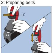
Separate belts by pressing buckle button C and while pulling apart
