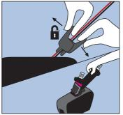
To release the passenger unlock the comfort clip. Disconnect burgundy strap from black belt and hold strap until its retracted into the reels to avoid whiplash. Repeat when unbuckling the black belt
