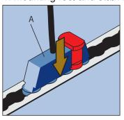
Mount the real and stalk devices by Inserting the Plunger Stud Fitting (A) into the floor tracking
