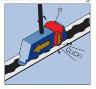
Slide the Plunger Stud Fitting until plunger B drops into a hole in the floor tracking. The device is now locked in the floor tracking
