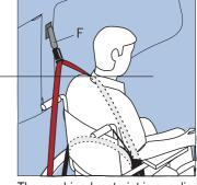
The combined restraint is supplied with an additional tongue on the shoulder belt and this should be used in conjunction with an extension belt F. If the occupant belt is too short, the extension belt clips into the inertia tongue and goes from the shoulder and locks into the vehicle wall.
