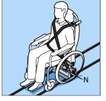
Repeat the previous using other all age inertia belt and fixing it into the lowest buckle N on the other side of the seat
