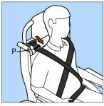
Position the age adjuster P (on both all age inertia belts) to ensure webbing does not cut across the occupants neck
