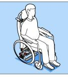
Unbuckle the passenger restraint seatbelts so the occupant is free being careful to hold the belts till fully retracted to prevent whiplash
