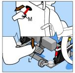
To release foot pedal L pull Rachet Release Webbing M whilst pressing down on foot pedal L then at the same time release foot pedal L gently allowing it to return to its uppermost position. Then let go of the red release webbing so the dogs are no longer engaged in the ratchet on the base
