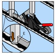
Use the round spigot E at the front of the seat legs (if available) to insert into the floor tracking holes.
