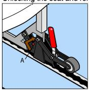
Lift safety bolt A to its upper position
