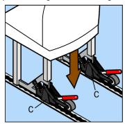
Lower the rest of the seat into the tracking. The Millennium Wheel Seat Fittings C should now sit in line with the tracking
