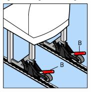
Rest on tracking and ensure handles B are unlocked by pointing away from the chair as shown above. If not please unlock them using the instructions in the next section
