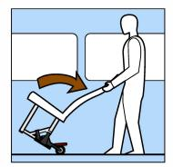
Using the wheels as a pivot point, lean the seat backwards out of the floor tracking. The seat should now be free of the tracking and can now be moved
