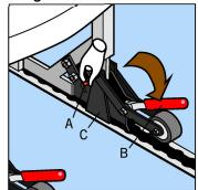
While holding safety bolt A in its upper position pull handles B away from the Millennium 2 Fitting C to unlock.
