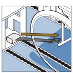
Extend the rear webbing retractor located on the rear
