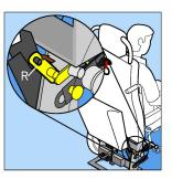
Lock the cushion on both sides by applying yellow tab R over the pin on the cushion squab
