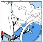
Pull the karabiners (K) from the front of the seat base and attach to the rear of the wheelchair frame as low down as possible on the wheelchair manufacturer's recommended securement points
