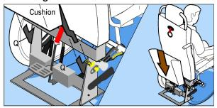
With the underside of the cushion facing the back support locate the protruding parts of the cushion into the brackets (Q) on the back of the
