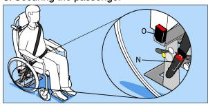
Secure the passenger using the two all age inertia belts. Take one belt and insert it into the lowest buckle N.
