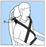
Position the all age adjuster P (on both belts) to ensure webbing does not cut across the occupants neck. Simply push down to just below shoulder level
