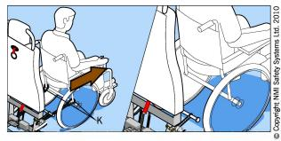
Disengage the wheelchair brakes and move the wheelchair forward
