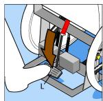
Press down on foot pedal L to tighten the webbing and secure the wheelchair. To ensure the correct webbing tension with no slack you may have to release the pedal and tread down several times. (See next image)
