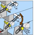
To adjust the adjustable adapter beam H to angle up or down to receive the wheelchair pull plunger I. While holding plunger I raise and lower H to your preferred angle then let go of I. I should snap in to lock the angle. (You may have to alter the angle of the beam to the closest point I will snap
