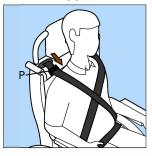
Position the all age adjuster P to ensure webbing does not cut across the occupants neck. Simply push down to just below shoulder level
