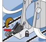
While holding safety bolt A in its upper position pull clamp B away from the Millennium 2 fitting C to unlock. The restraint device is now unlocked and can be inserted into the floor tracking
