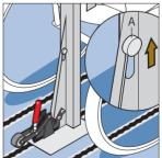
To unlock the Millennium Fitting either to prepare it to insert it into the tracking or to remove the Saferider lift bolt A
