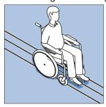
Position the wheelchair where the tracking is set at the measured centres
