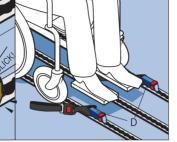
The devices (D) are now locked in the floor tracking
