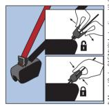
Note: Where the upper belt mount sits slightly too high above the shoulder (due to wheelchair handlebars) use wheelchair handlebars) use the comfort clip located on the burgundy diagonal belt. Simply pull out the webbing to allow some slack then click the comfort clip together.
