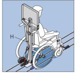
Position the Saferider millock H in the centrally positioned track behind the wheelchair and insert it into the tracking. See Note 1 below to insert the Saferider into the tracking
