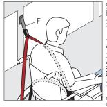
If the combined restraint is supplied with an additional tongue on the shoulder belt then this should be used in conjunction with an extension belt F. Where applicable, the extension belt clips into the inertia tongue and goes from the shoulder and locks into the vehicle wall. (Note: Only applicable if not using Saferider)
