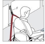
If the combined restraint is supplied with an additional tongue on the shoulder belt then this should be used in conjunction with an extension belt F. Where applicable, the extension belt clips into the inertia tongue and goes from the shoulder and locks into the vehicle wall. (Note: Only applicable if not using Saferider)
