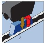
Mount the real and stalk devices by Inserting the Plunger Stud Fitting (A) into the floor tracking (Install the straps device with the strap with tongue nearest to the rear of the wheelchair)
