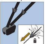
Unlock comfort clips by pulling the two larger ends apart.
