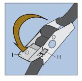
Close I till H engages so the strap becomes fixed. Repeat tensioning process on other side of wheelchair to secure it. The wheelchair should not be able to move
