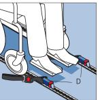
Lock Plunger Stud Fittings D (see Note 1 on next page to see how to do this) of Fixed Straps into tracking in front of the wheelchair
