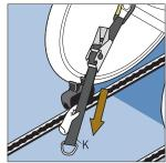
Pull loose ended strap K till webbing is tight and so strap in front of the wheelchair is also in tension
