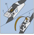
To make the belt adjustable push in H of I and rotate I to the other end
