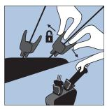
To release the passenger open comfort clip on both straps. Unclip clip and latch and hold shoulder strap until it retracts into the reels to avoid whiplash. Release strap from stalk buckles and hold belt as before till fully retracted
