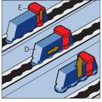
To remove front fixed strap Plunger Stud Fittings pull up Plunger E, slide Plunger Stud Fitting D till the unit aligns with the holes in the track. When aligned the device can be lifted out
