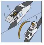
To make the rear wheelchair straps adjustable push in H of I and rotate I to the other end. The karabiners can now be removed from the wheelchair. At the front of the wheelchair press buckle buttons on fixed straps to release tongues
