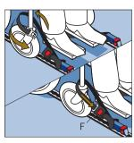
Wrap around appropriate attachment point on front of wheelchair and reconnect with buckle F. Repeat process on other side of wheelchair
