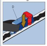
Attach the webbing devices to the floor by Inserting the Plunger Stud Fitting (D) into the floor tracking
