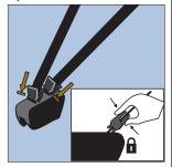
Once clips are at the bottom they can be locked by pushing the two larger ends together. These will make the belt straps feel less tight for the user
