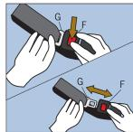
Separate belt tongue G and buckle by pressing button F while pulling apart
