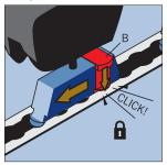
Slide the Plunger Stud Fitting until plunger B drops into a hole in the floor tracking. The device is now locked in the floor tracking
