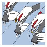
Separate the belts by releasing clip C from latch D
