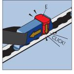
Slide the Plunger Stud Fitting until plunger E drops into a hole in the floor tracking. The device is now locked in the floor tracking
