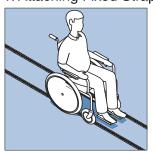
Position the wheelchair where the tracking is set at the measured centres of 330mm
