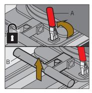
If you wish to change the seat's position unlock the seat base by lifting up red toggle clamp A to the upright position. Then lift handle B to raise the plunger out of the hole.
