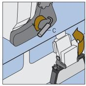
Push down handle on the side of the seat and rotate the whole seat so the back faces the wall. It should click into position and should not be able to move.
