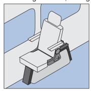
To return the seat to it's seat position reverse the steps above. Ensure the chair is slid forward far enough that the wheel arch does not get in the way of the passenger's legs.
