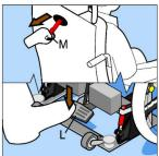
To release foot pedal L pull Rachet Release Webbing M whilst pressing down on foot pedal L then at the same time release foot pedal L gently allowing it to return to its uppermost position. Then let go of the red release webbing so the dogs are no longer engaged in the ratchet on the
