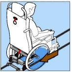
Bring the wheelchair up against the adapter beams and seat back. Armrests on the seat back can be rotated out of the way if needed
