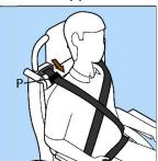
Position the all age adjuster P to ensure webbing does not cut across the occupants neck. Simply push down to just below shoulder level
