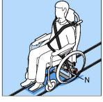
Repeat the previous using other all age inertia belt and fixing it into the lowest buckle N on the other side of the seat
