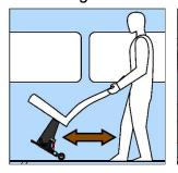
Tilt the seat back and use the wheels to roll seat into correct position over the tracking
