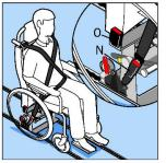
Secure the passenger using the two inertia belts. Take one belt and insert it into the lowest buckle N. Repeat using the other inertia belt and fixing it into the lowest buckle on the other side of the seat. Note: Where necessary use extension belts provided
