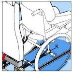
Pull the karabiners (K) from the front of the seat base and attach to the rear of the wheelchair frame as low down as possible on the <u>wheelchair</u> <u>manufacturer's recommended</u> <u>securement points</u>
