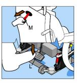
To release foot pedal L tread on it and pull the red rachet release webbing M. Then take your foot off the pedal and let it go up to its uppermost position whilst still holding the webbing. Then let go of M
