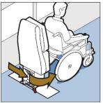
Slide and rotate the seat to align with the back of the wheelchair
