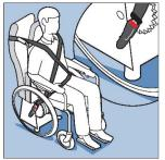
Secure the passenger using the two all age inertia belts. Take one belt and insert it into the buckle. Repeat using the other all age inertia belt and fixing it into the buckle on the other side of the seat
