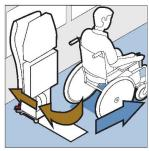
Rotate and slide the seat base to the side. The wheelchair user can now pass.
