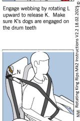
Position the age adjuster N (on both all age adjuster belts) to ensure webbing does not cut across the occupants neck
