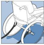
Attach the karabiners to the rear of the wheelchair frame as low as possible on manufacturer's recommended points
