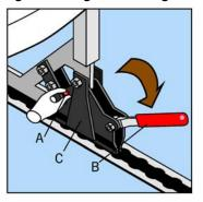
While holding safety bolt A in its upper position pull handles B away from the Millennium 2 fitting C to unlock. Repeat on other leg. The seat is
