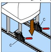
Insert the Millennium 2 Seat Fitting C into the tracking.
