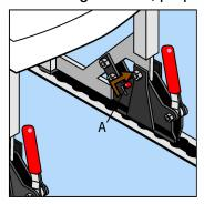
Align the seat legs resting them on the floor tracking. Lift safety bolt A to its upper position
