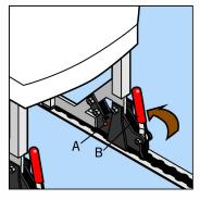
Close handles B to lock the chair in its new position. The safety bolts A should rest in their lower position. Repeat on other leg. The chair is now secure
