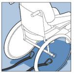
Release wheelchair brakes (+ switch on electric versions). Move the wheelchair forward to extend the webbing belt restraints. Put on the brakes (+ switch off power) and remove the webbing belt karabiners
