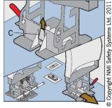
Lift the drop lock C at the back of the seat and slide the seat base forward off the floor pocket
