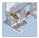
Slide the seat base onto the raised floor pocket
