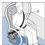
Now assist and apply the inertia belt O located on the seat back around the wheelchair passenger
