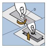
Raise the floor pocket closest to one you just closed by turning D to align with the dot and then pulling it up
