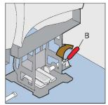
Unclamp wall seat by turning clamp handle B away from the seat
