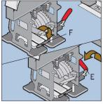
Drop safety latch F and clamp E by pointing the clamp handle towards the seat base
