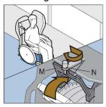
Assist the wheelchair user if necessary to remove their seatbelt. Remove any support cushion. To release the webbing belts rotate safety catch N from back of M. Push M as far as it will go and rotate N so it holds M in up position
