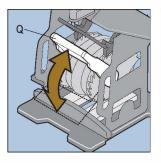
Pump foot pedal Q with foot to rachet in the wheelchair until the wheelchair is secure Note: Do not over tighten
