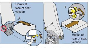
To remove the seat squab locate the release hooks. Both of these are either located on each side of the seat (Left image) or on some models at the back (Right image). Pull out plunger A from the hole on both sides of the seat and rotate hooks upwards and remove the seat squab and store. Repeat on other seat
