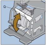
Pump the foot pedal Q to rachet the webbing belts onto the webbing drums. Do not over tighten
