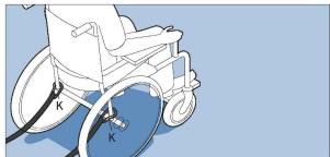
Attach the karabiners (K) to rear of the wheelchair frame as low down as possible on manufacturer's recommended securement points
