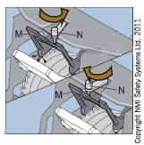
To engage the webbing drums rotate hook N away from dog arm M so M is released and the dogs engage with the ratchet drums. Then rotate safety catch N behind M.
