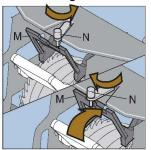
To release the webbing belts rotate safety catch N from back of M. Push M as far as it will go and rotate N so it holds M in the upper position
