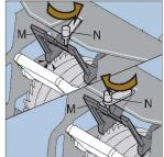
To engage the webbing drums rotate hook N away from dog arm M so M is released and the dogs engage with the ratchet drums. Then rotate safety catch N behind M.
