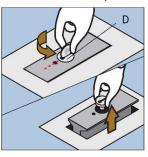
Raise the floor pocket nearest the wall by turning D to align with the dot and then pulling it up
