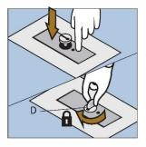
Push down the remaining floor pocket and lock in lower position by pushing in D and turning 90° away from the alignment of the dot
