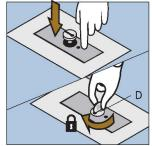
Push down the raised floor pocket and lock in lower position by pushing in and turning D 90° away from the alignment of the dot
