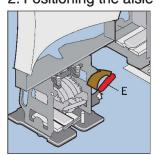
Unclamp wall seat by turning clamp handle E away from the seat
