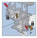
Lower drop lock C and clamp to lock by turning the clamp handle B towards the seat. The side seat is now in the side position
