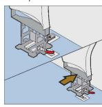
Slide wall seat base onto the raised floor pocket
