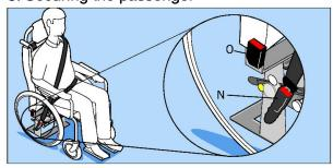
Secure the passenger using the two all age inertia belts. Take one belt and insert it into the lowest buckle N.
