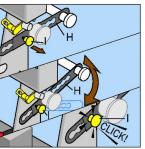
To adjust the adjustable adapter beam H to angle up or down to receive the wheelchair pull plunger I. While holding plunger I raise and lower H to your preferred angle then let go of I. I should snap in to lock the angle. (You may have to alter the angle of the beam to the closest point I will snap
