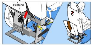
With the underside of the cushion facing the back support locate the protruding parts of the cushion into the brackets (Q) on the back of the seat
