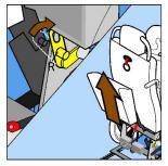
Remove seat cushion from the back of the wheelchair by lifting off yellow tabs (R) from both sides of the seat and then lifting the cushion out
