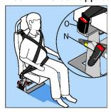
Secure the passenger using the two all age inertia belts. Take one all age inertia belt and insert it into the highest buckle O. Repeat using other inertia belt and fixing it into the highest buckle on the other side of the seat
