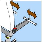
Slide the adjustable bars to align them with the required position to accept the wheelchair
