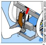
Now tread on pedal again to eliminate slack in the webbing. Put wheelchair brakes on and check wheelchair is secure
