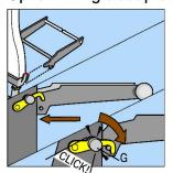
If you have the rigid adapter beam version locate it into the location points that the seat cushion frame was originally located in. Rotate yellow hook down to engage with the adapter beam and make sure plunger G engages by locking the hook in position. Repeat on the other side of the seat
