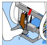
Press down on foot pedal L to tighten the webbing and secure the wheelchair. To ensure the correct webbing tension with no slack you may have to release the pedal and tread down several times. (See next image)
