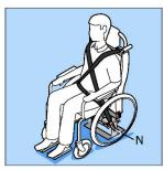
Repeat the previous using other all age inertia belt and fixing it into the lowest buckle N on the other side of the seat
