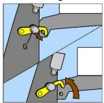
To remove the seat cushion pull out plunger G on the yellow hooks on both sides of the seat frame and rotate hooks upward
