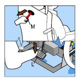
To release foot pedal L tread on it and pull the red rachet release webbing M. Then take your foot off the pedal and let it go up to its uppermost position whilst still holding the webbing. Then let go of M
