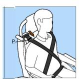
Position the age adjuster P (on both all age inertia belts) to ensure webbing does not cut across the occupants neck
