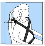
Position the all age adjuster P (on both belts) to ensure webbing does not cut across the occupants neck. Simply push down to just below shoulder level
