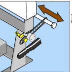
The adjustable bars can be slid to the appropriate position to meet the wheelchair frame. Repeat on the other side of the
