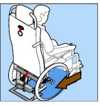
Bring the wheelchair up against the adapter beams and seat back. Armrests on the seat back can be rotated out of the way if needed
