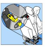
Lock the cushion on both sides by applying yellow tab R over the pin on the cushion squab frame
