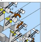
To alter the length of adapter beam H pull out plunger J and rotate 90°. Slide beam H to vour required length then turn back J so the marks line up with the length of the beam. J should click back into place to lock, if it does not adjust the length of H slightly till it does. Repeat on the other side of seat base
