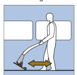
Tilt the seat back and use the wheels to roll seat into correct position over the tracking
