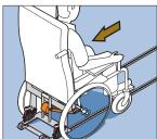
Reverse the wheelchair against the seat back. Ensure the adjustable bars are against the frame
