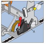
Close handle B to lock the seat back in its new position. The safety bolts A should automatically drop and rest in their lower position. Repeat on other leg
