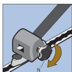
Finally, remove any slack and tighten the restraint by turning the knob N on the side.
