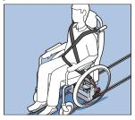
Repeat the previous step using the other all age inertia belt and fixing it into the opposite buckle on the other side of the seat
