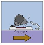
Once in the track slide the unit forward till L drops fixing the unit in position
