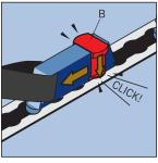
Slide the Plunger Stud Fitting until plunger B drops into a hole in the floor tracking. The device is now locked in the floor tracking
