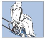
Secure the passenger using the two all age inertia belts. Take one all age inertia belt and insert it into the opposite buckle
