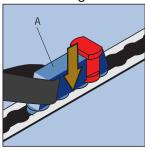
Front belts: Insert the Plunger Stud Fitting (A) into the floor tracking
