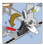
While holding red safety bolt A in its upper position pull clamp B away from the Millennium 2 fitting C to unlock. Repeat on other leg
