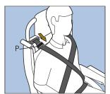
Position the age adjuster P (on both shoulder straps) to ensure webbing does not cut across the occupants neck
