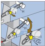
To adjust the adjustable adapter beam H to angle up or pull plunger I. While holding plunger I raise and lower H to of I. I should snap in to lock the angle. (You may have to alter the angle of the beam to the closest point I will snap
