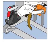
Ratchet the wheelchair in tight by holding main handle J and moving it up and down. When webbing is secure lower handle J to its lowest position
