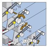
To alter the length of adapter beam H pull out plunger J and rotate 90°. Slide beam H to your required length then turn back J so the marks line up with the length of the beam. J should click back into place to lock, if it does not adjust the length of H slightly till it does. Repeat on the other side of seat base
