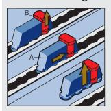
To remove pull up Plunger B, slide Plunger Stud Fitting A till the unit aligns with the holes in the track. When aligned the device can be lifted out
