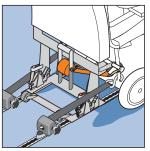
Connect the webbing to the back of the wheelchair as low down as possible on the wheelchair manufacturer's recommended securement points
