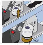
Lift and turn the grey plunger (E) so the lines on the plunger are turned 90° from the direction of the tracking. Repeat on other side. The seat back is now unlocked
