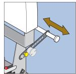
The adjustable bars can be slid to the appropriate position to meet the wheelchair frame. Repeat on the other side of the seat
