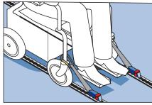
Attach the karabiners to the front of the wheelchair. Connect as low down as possible on the <u>wheelchair manufacturer's recommended securement points.</u> You may need to move the fixings in the floor to reduce slack
