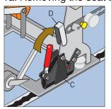
Unlock the Millennium 2 Fitting C by removing guard D. Repeat on other leg
