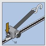
Press down M and disconnect the hooks from the wheelchair. Holding down M will let the restraint retract
