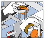
To open the ratchet squeeze bar H to unlock and lift handle J up and forward to uppermost point and then let go
