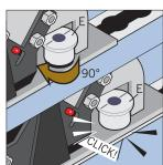
Locate the Millennium Fittings in the track. Turn the plungers E on both sides of the seat so the lines are parallel with the tracking. Move the unit slightly backwards and forwards till the plungers drop into the track hole
