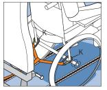
Pull the karabiners (K) from the front of the seat base and attach to the rear of the wheelchair frame as low down as possible on the <u>wheelchair</u> <u>manufacturer's recommended</u> <u>securement points</u>
