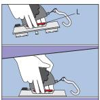
Lift L to drop the retractable restraints into the track
